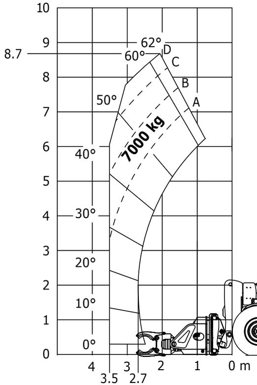
Machine on tyres with CH10-4 tons
